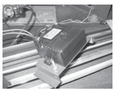
Connect the ground wire to the DC Sparker mounting bracket.
